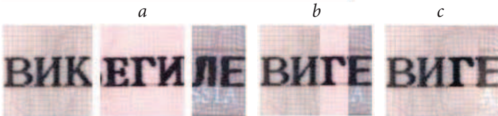
Fig. 7. Bonding of the images' fragments: a – original image slices; b – the result of a “naive” gluing images; c – the result of the “seamless” gluing of the images [7].
