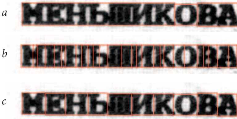
Fig. 10. The example of the second work stage of the algorithm: a – initial cross-sections; b – the result of the two groups of cross-sections combination; c – the final result of segmentation.
