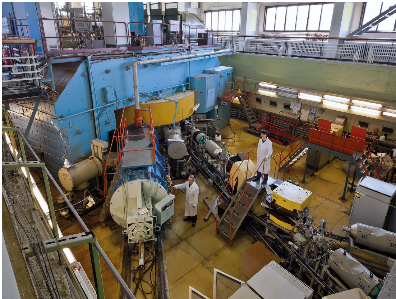
Fig. 1. Heavy ion accelerator U-400 of Flerov Laboratory of Nuclear Reactions JINR.
