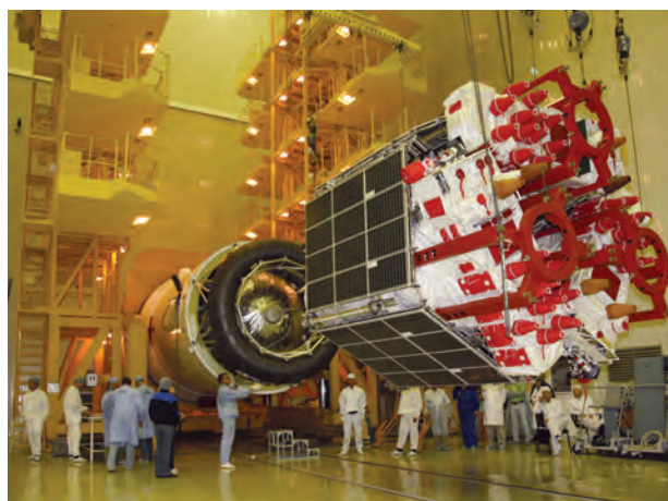
Fig. 10. SC "Glonass-M": docking of a block of three spacecrafts with an upper stage at the cosmodrome.
