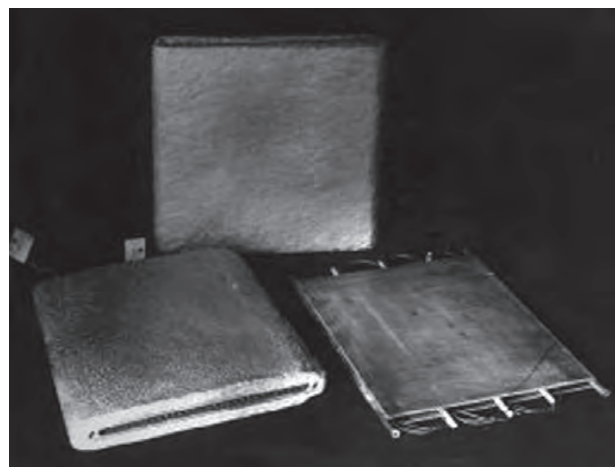
Fig. 2. Test samples of molded insulation with a coating, which are intended to be tested at temperatures of 1500–2200 °C.
