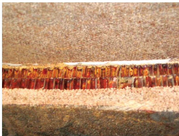
Fig. 1. Cross-section view of the spacecraft "Vostok-1" thermal protection.
